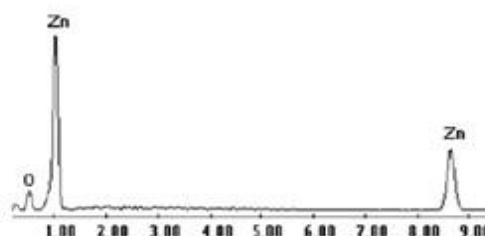
Figure 1. Elemental analysis (chemical composition) of zinc oxide (ZnO) nanoparticles by energy dispersive X-rays (EDX)
