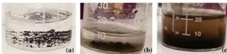
Figure 6. General appearance of chitin extracted by (a) alkaline, and enzymatic treatment, (b) before and (c) after ultrasonication process. [Color figure can be viewed at wileyonlinelibrary.com ]
